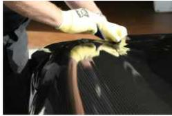
**Surface #3** - The bottom portion, Surface #3 is where it get fun. Being by pulling the vinyl out, and then down. use your hand to conform the material. Pull to conform toward the front, over the headlight well. Squeegee toward your pressure hand, moving air forward. Apply heat to conform around headlight well. After heating, use your
