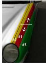
**Surface #2** - For the top area, squeegee horizontally left to right, applying beyond your intended area of application well past the seam between the hood and fender.
